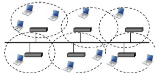
Fig-2 (Wireless Network Structures-II (Infrastructure less Networks))
